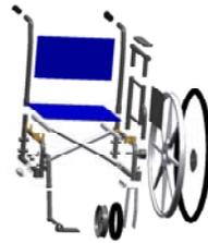
**Figure 4:** Exploded view of most manual wheelchair generic parts.
