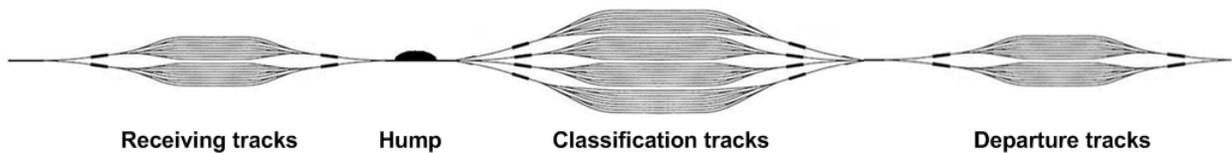
Figure 1: The generic structure of a hump yard
