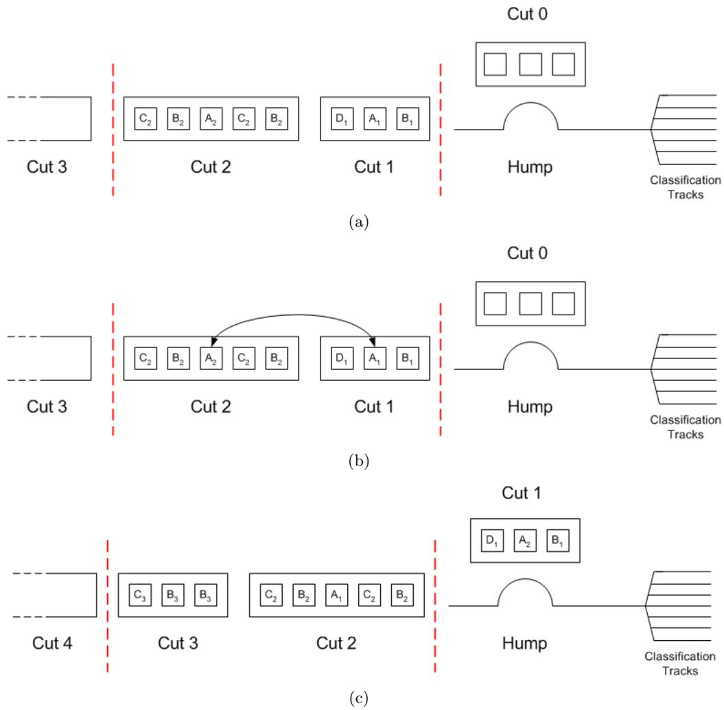
Figure 3: Illustration of the the sliding time window procedure with (a) Cut 0 being humped (b) Swapping operation takes place inbetween Cuts 1 and 2 (c) Cut 1 being humped
