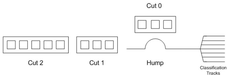
Figure 2: Illustration of the humping process and the cut queue
