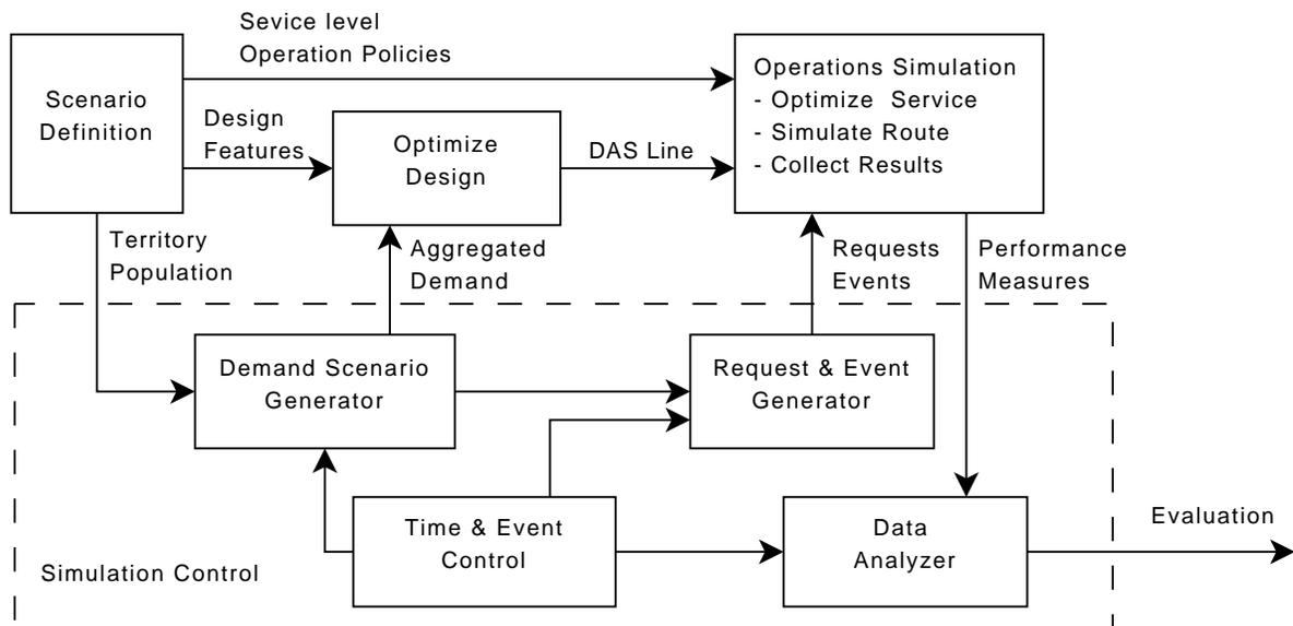
Figure 2: Evaluation Framework for a DAS Line
