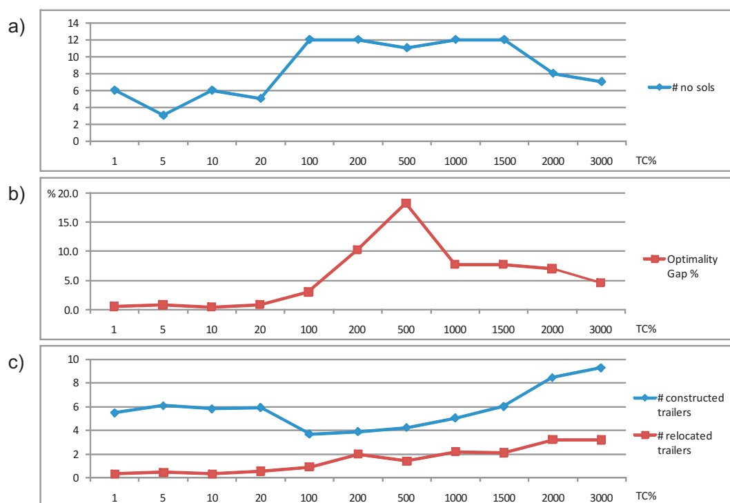
Figure 3: The impact of the transportation cost ratio on (a) the number of CSLP instances where no solutions have been found, (b) the average optimality gaps and (c) the average number of constructed and relocated trailers in near optimal solutions.
