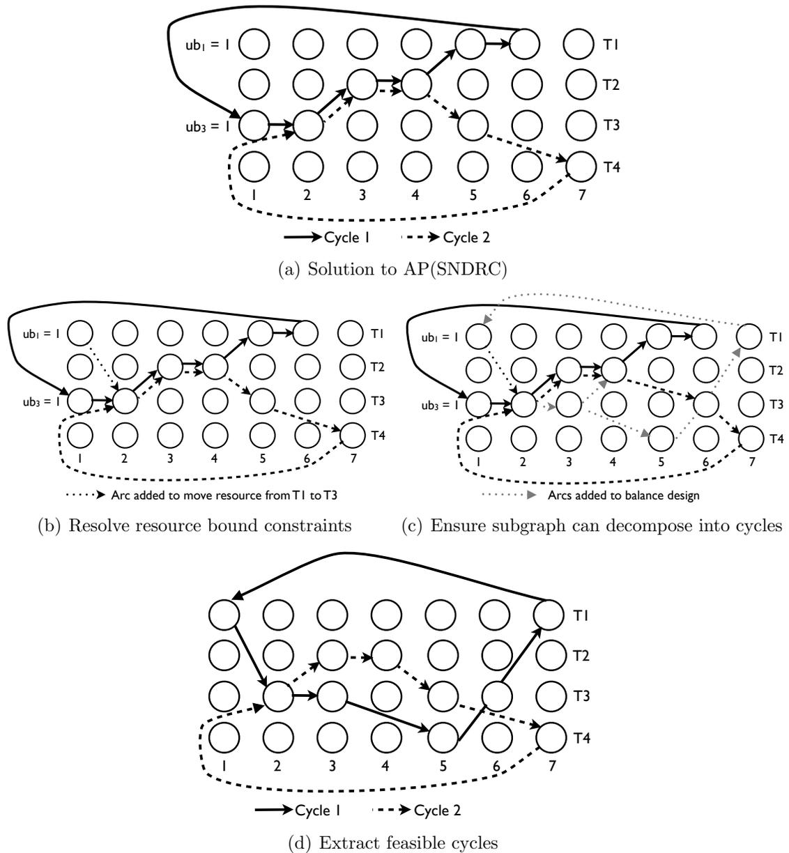
Figure 5: Converting a solution to AP(SNDRC) to a solution to SNDRC
