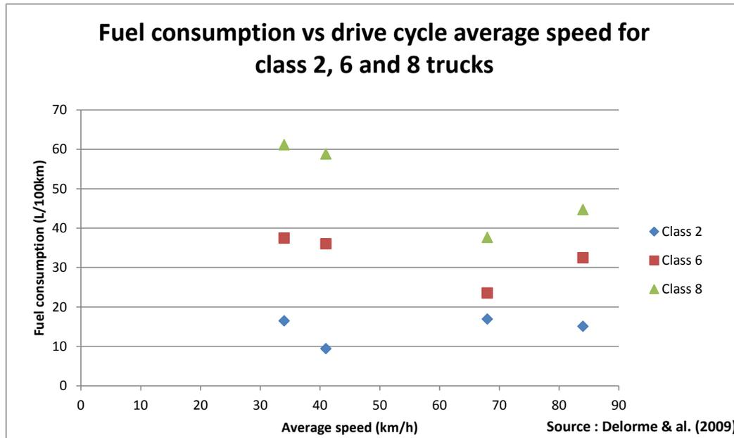
Figure 4: Fuel consumption vs. drive cycle average speed for class 2, 6 and 8 trucks
