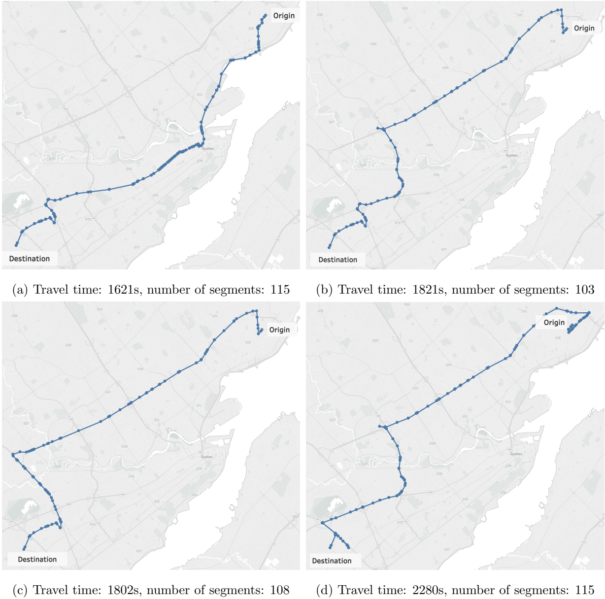
Figure 4: Optimal time-dependent travel times and number of segments for the same origin-destination, across different starting times (see Table 2)
