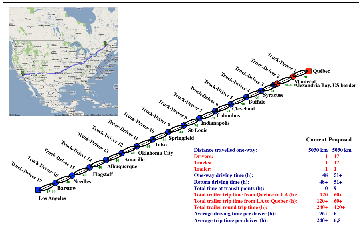
Figure 2. Contrasting current point-to-point transport and Physical Internet enabled distributed transport
