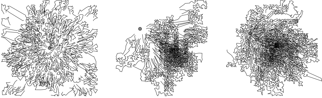
Figure 10: Solutions for the new instances based on parcel distribution in Belgium: Antwerp (central depot), Ghent (edge depot), and Brussels (edge depot). The edges connected to the depot are not displayed.
